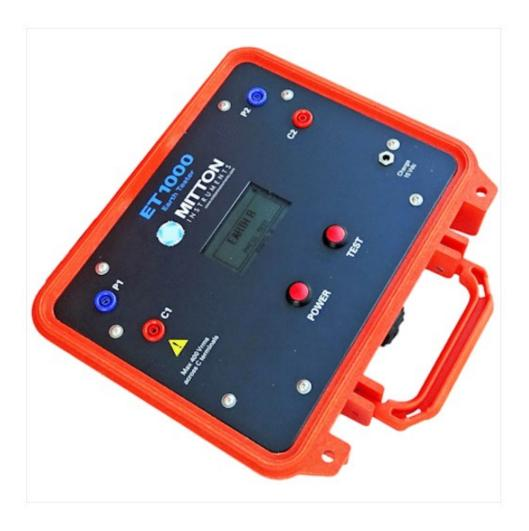
The ET1000 is a versatile 4-terminal earth tester suitable for the measurement of soil resistivity, earth electrode or grid resistance, conductor/joint resistance and primary plant bonding resistance.
